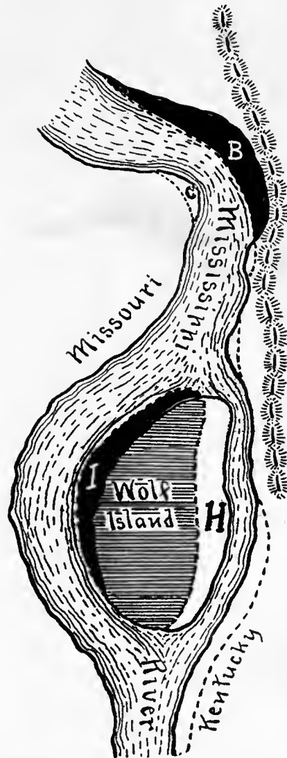
Historic case in which treaties between France, Spain and England were changed by the shifting of a great river channel which altered the boundaries between Missouri and Kentucky—Continuous lines represent original banks of river—Dotted lines represent present banks—Land marked B is new timberland—Land marked C is boundary point that is washed away—Land marked H is strip of Wolf Island that has been washed away—Land marked I shows accretions on western side of Wolf Island—Map drawn for historical record in THE JOURNAL OF AMERICAN HISTORY
